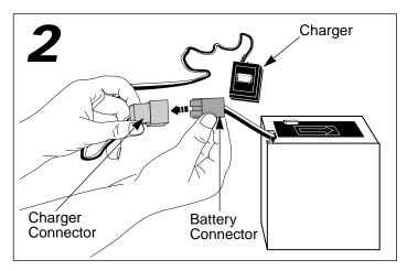
• Plug the charger and battery connectors together. **IMPORTANT NOTE!** If you are recharging your battery, you will first need to disconnect the battery connector from the motor harness connector under the seat.
